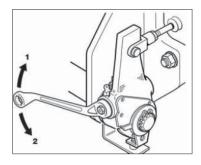
12. Check that the ASA is functioning by applying the brakes a few times. The ASA is working when the hex nut rotates clockwise on the return stroke.
