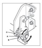
10. Rotate the anchor bracket assembly to align the anchor screw with the slot in the control arm. Tighten the anchor screw. While insuring that the control arm does not move out of position, as set in item 9, tighten the anchor bracket clamp bolt, thus fixing the anchor bracket to the camshaft tube. A minimum of 1/16" should protrude through the control arm as illustrated.
