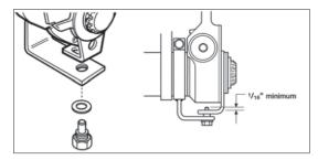
Adjust the clearance by rotating the hex nut on the ASA clockwise
