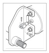
3. Loosely install the anchor bracket around camshaft tube. Do not tighten at this time.
