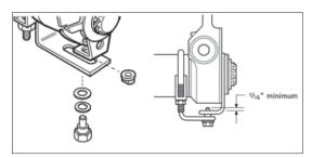
11. Adjust the clearance by rotating the hex nut on the ASA clockwise (1) until the brake lining touches the brake drum, then back-off by rotating the hex nut a 3/4 turn counterclockwise (2) Backing-off produces a loud clicking noise.
