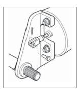
3. Loosely install U-bolt and anchor bracket saddle around camshaft tube. Do not tighten at this time.
