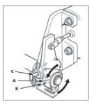
10. Install anchor screw, washers and slide nut to engage with the control arm slot. Tighten anchor screw to slide nut. While insuring that the control arm does not move out of position, as set in step 9, tighten the U-bolt anchor bracket to the camshaft tube. A minimum of 1/16" should protrude through the control arm as illustrated.
