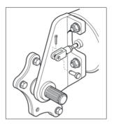
3. Attach the anchor bracket to the spider using the existing washers and bolt. Do not tighten at this time.
