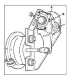
10. Install anchor screw, lockwasher, flat washer and slide nut into anchor bracket assembly and finger tighten. While insuring that the control arm does not move out of position, as set in step 9, engage the anchor screw in the control arm and tighten the spider bolt to the spider. Tighten the anchor screw to 20 ft.lbs. A minimum of 1/16" should protrude through the control arm and a minimum of 1/16" must be maintained between the slide nut and the control arm as illustrated.
