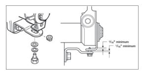
11. Adjust the clearance by rotating the hex nut on the ASA clockwise (1) until the brake lining touches the brake drum, then back-off by rotating the hex nut a 3/4 turn counterclockwise (2) Backing-off produces a loud clicking noise.
