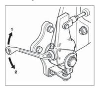
12. Check that the ASA is functioning by applying the brakes a few times. The ASA is working when the hex nut rotates clockwise on the return stroke.
