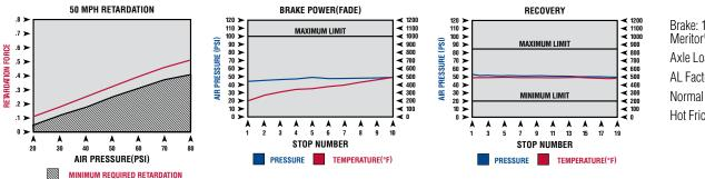
Brake: 16 1/2" x 7" Meritor® S-Cam Axle Load: 23,000 lb AL Factor: 165 Normal Friction: .429 F Hot Friction: .445 F
