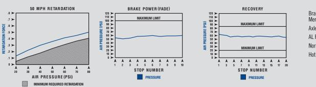
Brake: 16 1/2" x 7" Meritor® S-Cam Axle Load: 23,000 lb AL Factor: 165 Normal Friction: .453 G Hot Friction: .485 G
