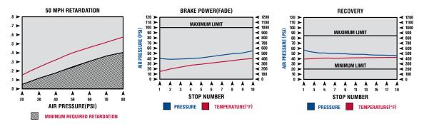
Brake: 16 1/2" x 8 5/8" Meritor<sup>®</sup> Cast Plus<sup>™</sup> Axle Load: 28,666 lb AL Factor: 195 Normal Friction: .463 G Hot Friction: .423 F
