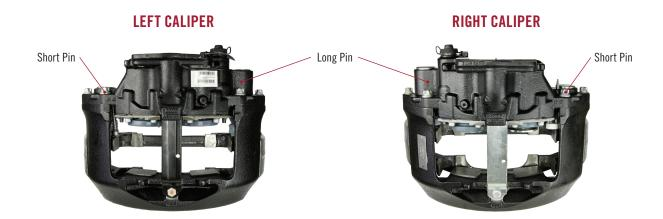
Calipers are right- or left-handed depending on where the long and short guide pins are located. To determine what type of caliper you have, position yourself at the front of the caliper and feel for the short slide pin side. If the short slide pin is in your right hand, it is typically a right (curb side) caliper.
