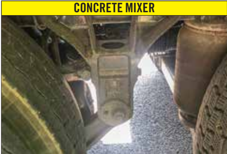
HENDRICKSON: PRIMAAX® The PRIMAAX features a square transverse beam connecting the two pivot beams connected the hangers. The hangers feature the Hendrickson logo and an alignment collar that features the Hendrickson logo. (pp. 76–77)
