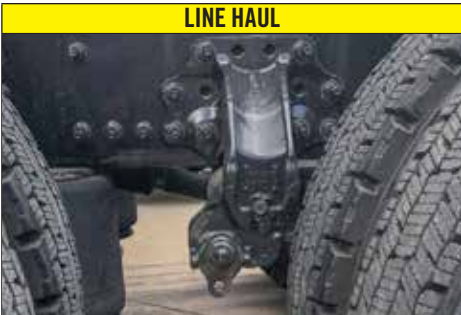
MACK® / VOLVO: CORPORATE AIR Identifiable by the unique hanger with a lower appendage that sits forward of the main body of the hanger. The genuine hanger typically has “Mack” or “Volvo” cast into the part. (pp. 20–21)
