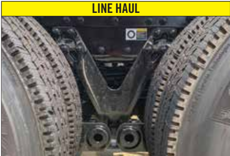
KENWORTH: AIRGLIDE 200® / 400® Newer version of the Kenworth 100. Identifiable by larger center hanger with two torsion bars connected at the bottom. The 200–400 series has a “V” cut out of the top of the hanger. (pp. 18–19)
