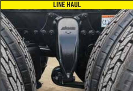
FREIGHTLINER: FAS II AIRLINER® Identifiable by the long thin solid hanger. The genuine hanger has “AirLiner” cast into the part. (pp. 14–15)
