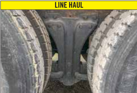
KENWORTH: AIRGLIDE 100® Identifiable by larger center hanger with two torsion bars connected at the bottom. This style of hanger is very unique to this suspension. (pp. 16–17)
