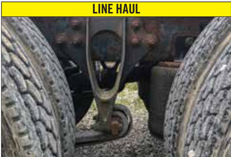
NAVISTAR / INTERNATIONAL®: CORPORATE AIR Identifiable by the long thin hanger with a hole cut out of the center. (pp. 22–23)
