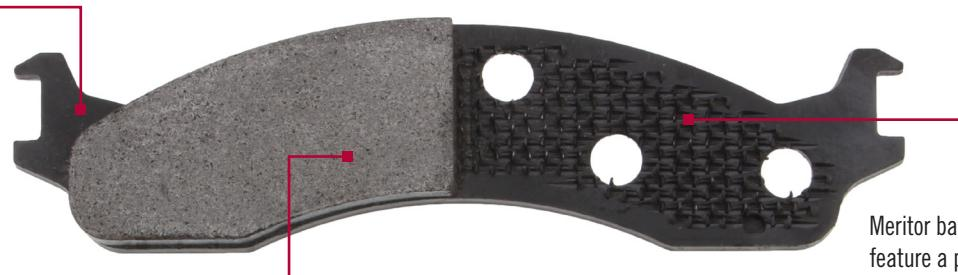
Meritor® hydraulic brake pads are manufactured with Level N material to meet 2025 less than 0.5% copper by weight compliance. Select Meritor hydraulic brake friction now with no need to change friction brands later to meet Level N 2025 standard.
