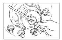
When performing periodic tire pressure checks, disconnect the tire hose from the hub cap connection. You do not need to turn off the system, as there is a check valve in the thru-t and one in the hose.
