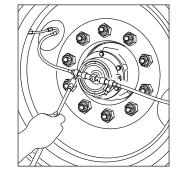
**NOTE:** Hoses equipped with the auxiliary check port (-CP) do not need to be removed from either end to check tire pressure. This can be done by applying a pressure gauge to the check port with the gator cap.
