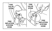
When the tire hose must be disconnected at the valve stem (for example, during a tire replacement), use the following guidelines for reattaching.
