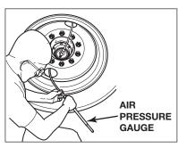
**NOTE:** Due to manufacturing variability of gauges, not all pressure gauges will fit the hub cap end of the hose. Dill Gauges SG-1 and SG-2 are compatible with PSI hoses. To order, contact Tuffy at tuffymfg.com or 800-341-6667.
