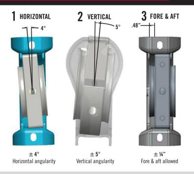
Dana Spicer® center bearing does not have the ability to adjust to three directions of misalignment as it does not allow for side-to-side and fore and aft misalignment, only vertical angularity.
