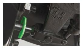
If the SimpleCheck disc travels beyond the end of the brake stud (as shown below), then further brake system diagnostics must be performed. It's that simple – and that fast.
