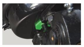
**How:** When the brake is applied (via service air pressure or parking brake spring pressure), the disc indicates how far the pushrod travels.
