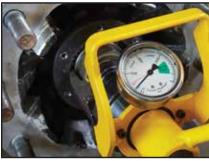
3. To set the bearings, loosen T-handle slowly until gauge pointer points to "Set Drive/Trailer Axle" or "Set Front Axle" accordingly.
