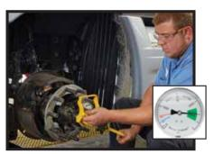
2. Seat the bearing rollers. Tighten T-handle to load the bearings until the gauge pointer is in green "Roll In Zone." Roll the wheel three revolutions.
