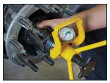
4. Finger-tighten the Temper-Loc nut against the bearing: align the closest dot on the nut to the key locator indicator mark.
