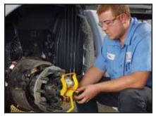
1. Attach Doctor Preload tool to end threads of the axle. Use a sweeping motion to guide the load arms around the locknut while engaging the key locator in the keyway. Engage the thread with two turns of thread with the end of the axle.
