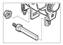
Adjust the clearance by rotating the hex nut on the ASA clockwise
