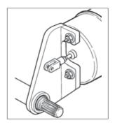
3. Loosely install U-bolt and anchor bracket saddle around camshaft tube. Do not tighten at this time.
