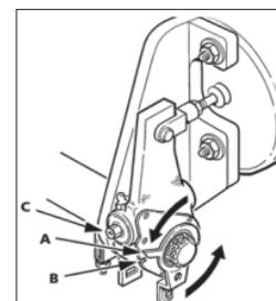
10. Install anchor stud into anchor bracket assembly and finger tighten using the 7/16" flange head nut. Position anchor stud in control arm slot. While insuring that the control arm does not move out of position, as set in step 9, tighten the U-bolt to the camshaft tube and anchor stud.
