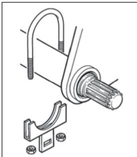
4. Coat the camshaft splines with anti-seize lubricant.
