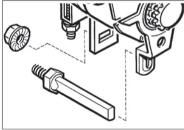
11. Adjust the clearance by rotating the hex nut on the ASA clockwise (1) until the brake lining touches the brake drum, then back-off by rotating the hex nut a 3/4 turn counterclockwise (2). Backing-off produces a loud clicking noise.
