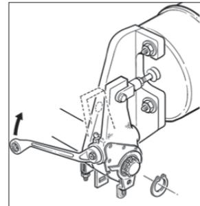
6. Wind the ASA into the clevis on the brake chamber piston rod by rotating the hex nut on the ASA in a clockwise direction until the hole in the ASA coincides with the holes in the clevis.
