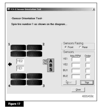
7. Follow the screen prompts, starting with 1, to rotate each sensed wheel end at a rate of 1/2 revolution per second. This rate equals a wheel speed of approximately 4 mph (7 kph). As each sensed wheel is rotated, check the color of the sensor identification block on the screen for results. Sensor identification boxes are located in the bottom left portion of the Sensor Orientation Test screen. Figure 16.
