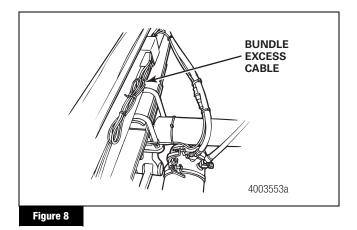
10. Secure excess cable in the sub-frame of the vehicle or along the air hoses as appropriate. Excess cable should not exceed two feet (0.61 meter).
