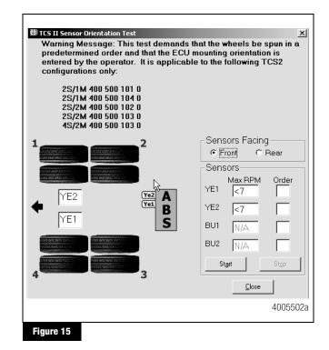
5. Click on *Front* or *Rear* in the *Sensors Facing* field to select the mounting orientation of the ECU/single modulator valve assembly.
