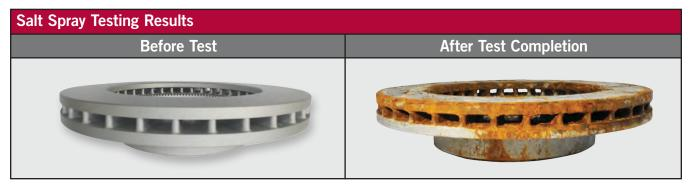
$<sup>^{\</sup>star}$  1,000 hours neutral pH salt spray testing per ASTM B117.
