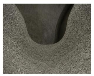
Contoured grain flow at the root enables higher fatigue life
