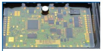
The WABCO ECU is fully potted, which provides a protective coating and safeguards against corrosion.
