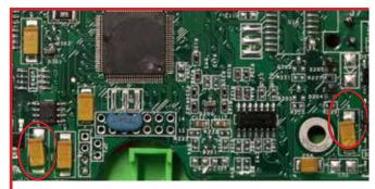
The ECU is not potted, which puts it at risk to corrosion and weakened performance over time.
