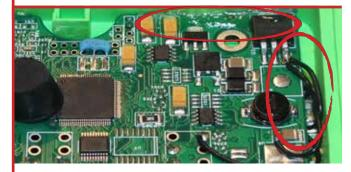
The PCB is not anchored to the ECU housing, but held with an inconsistent adhesive application, which provides minimal protection of PCB integrity.
