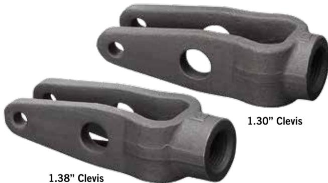
Meritor ASAs are sold in the aftermarket less clevis which allows the end user to properly spec the clevis for the intended application. Meritor manufactures clevises with pin spacings of 1.30" and 1.38" to accommodate a variety of applications. To maximize brake lining life, it is recommended to replace the clevis when the ASA is replaced.
